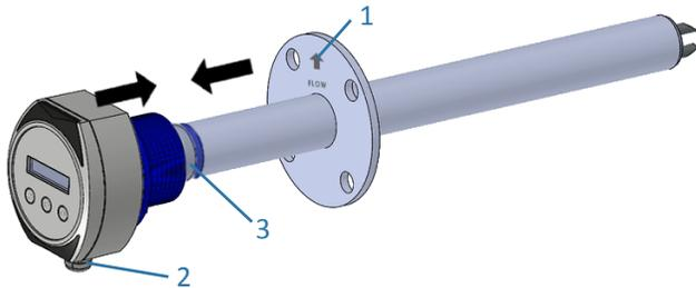
7c. Using a 10mm socket (or spanner) tighten clamp (3) to secure the head housing in position; torque to 5Nm.
