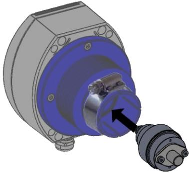
7b. Ensuring clamp (3) is fitted over the head housing shoulder and with the flow direction arrow (1) pointing upwards, carefully slide the probe body into the head housing (cable gland (2) at the base of the housing should face downwards).
