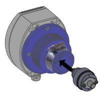
**7b.** Ensuring clamp (3) is fitted over the head housing shoulder and with the flow direction arrow (1) pointing upwards, carefully slide the probe body into the head housing (cable gland (2) at the base of the housing should face downwards).
