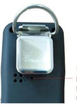
Pushing reset button through a hole on back of shell
