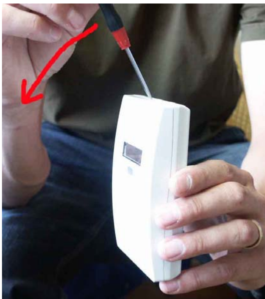
Figure 2. Closed housing seen from the side. The housing is opened by inserting a screwdriver and pushing left (to the front side).
