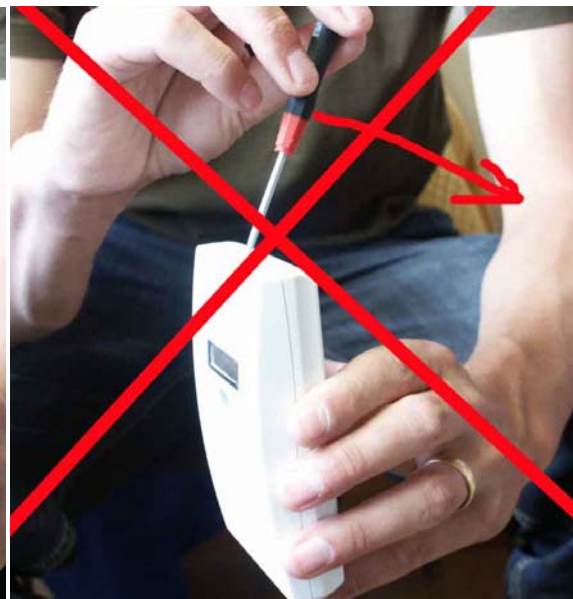
Figure 3. Closed housing seen from the side. Never push to the right. The locking hooks may break and damage the housing.
