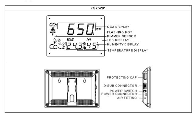
Dimmer function: When the light indoor become dark, the LED display will also become dark, then it can save power. NGC Function: When the switch of "NGC Function" is on, ZGkb301/ZGkb201 will enter into the Nature Gas Calibration mode.(NGC Function is not available in designated area)
