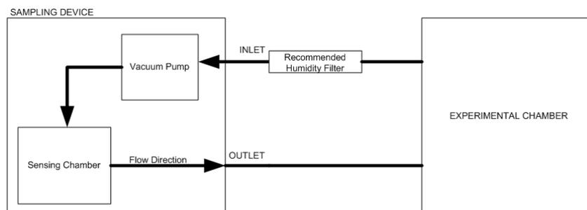
*Figure 4: Closed-loop operation*
