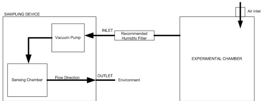
**Figure 5: Opened-loop operation**
