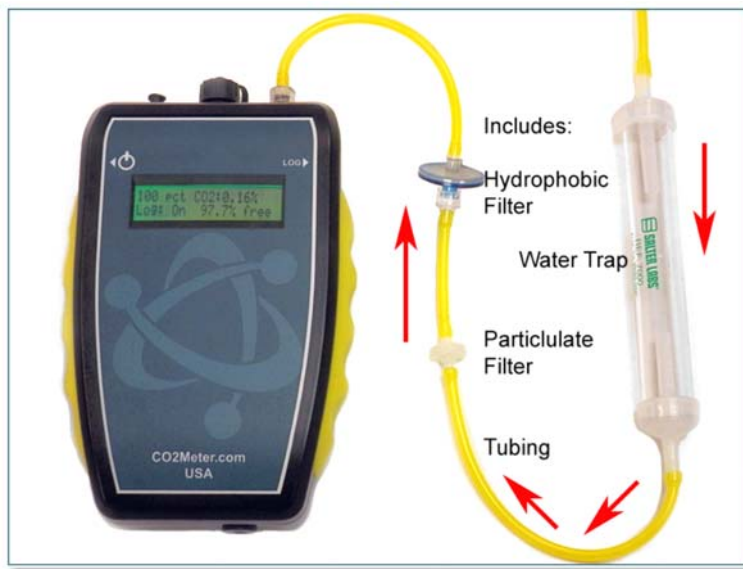
Figure 6: Filter Installation and Orientation
