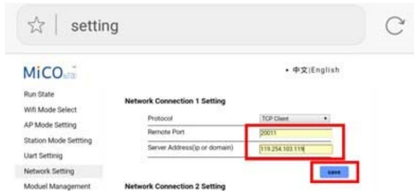
10. On the right side of the interface, select "Network Setting", and in the interface, for "protocol" click and select "TCP Client" and "save". The same do not restart the module.
