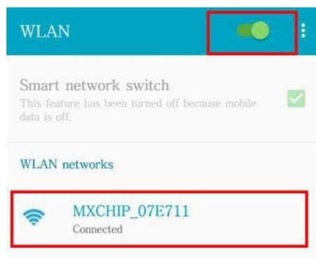
Note: researched WIFI hotspot is like MXCHIP\_07E711, MXCHIP\_ is an invariant format, 07E711 is a unique serial number for a WIFI module. Different WIFI modules have different serial numbers. It will be shown on the surface of the WIFI module.
