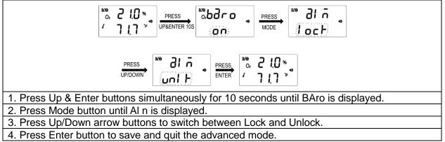
**9.2 Latch Function On / Off:** If the Latch function is on, alarms will continue until the reset button is pressed even if the O2 level returns to normal. Factory default is on.
