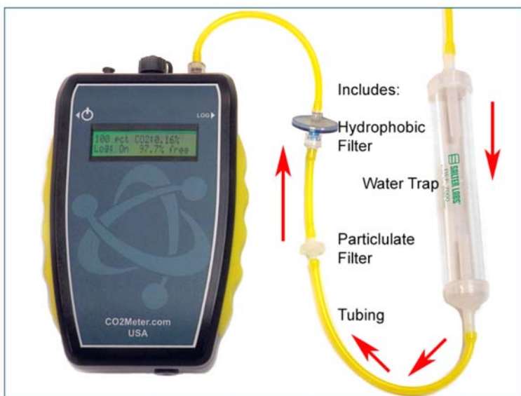
Figure 6: Filter Installation and Orientation
