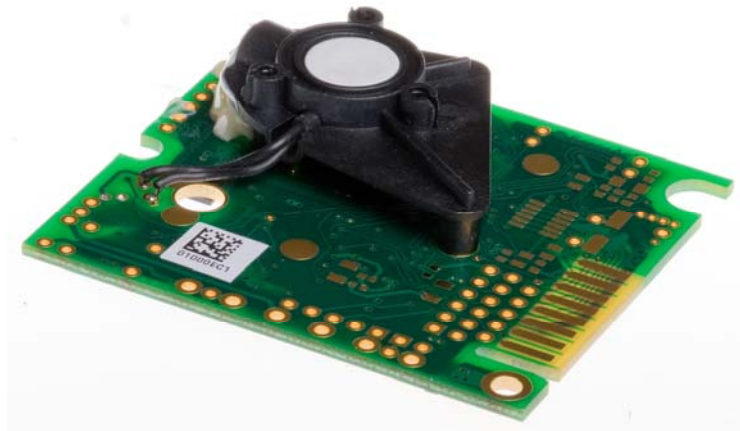
Figure 6. CO 2 Engine™ ICB diffusion model.
