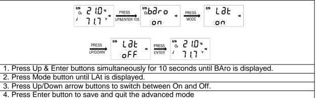
**1.3 Barometric Compensation On / Off**: Turns on automatic compensation for barometric pressure / altitude. Factory default is on.
