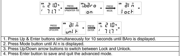
**1.2 Latch Function On / Off:** If the Latch function is on, alarms will continue until the reset button is pressed even if the O2 level returns to normal. Factory default is on.
