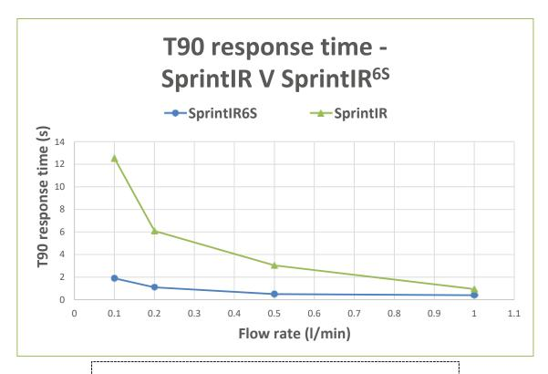
T90 time measured from 0 to 10% CO<sub>2</sub>. Digital filter switched off.
