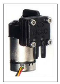
These pumps are constructed from molded, glass filled nylon with stainless steel tubing connectors and a brushless drive motor. They are fitted with Nitrile / Silicon diaphragm and valves. The pump uses efficient push-fit connectors designed for 2.4mm bore flexible tubing.
